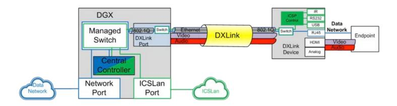
The Ethernet port on the DXLink device may disabled, or assigned to either the ICSLAN or the enterprise network.
